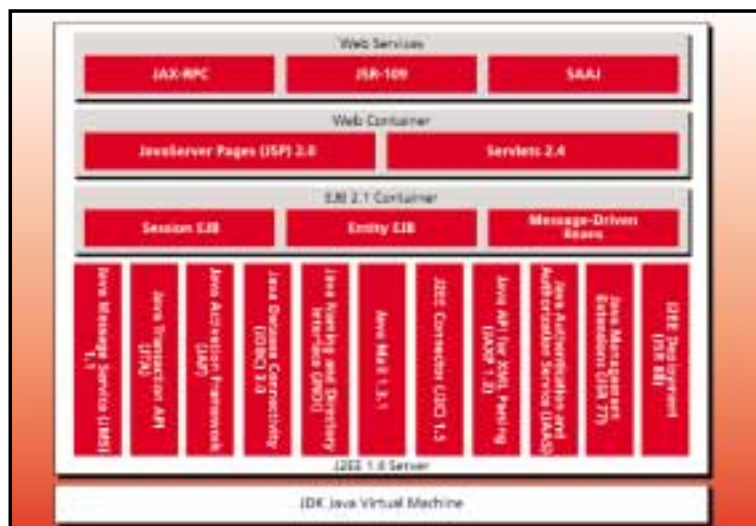
Figure 2 • Typical J2EE 1.4 server and its services
